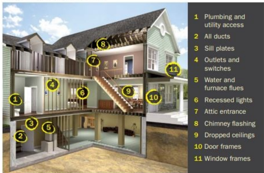
Where to Air Seal in a Home
